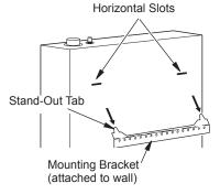
Figure 11 - Mounting Heater Onto Mounting Bracket
